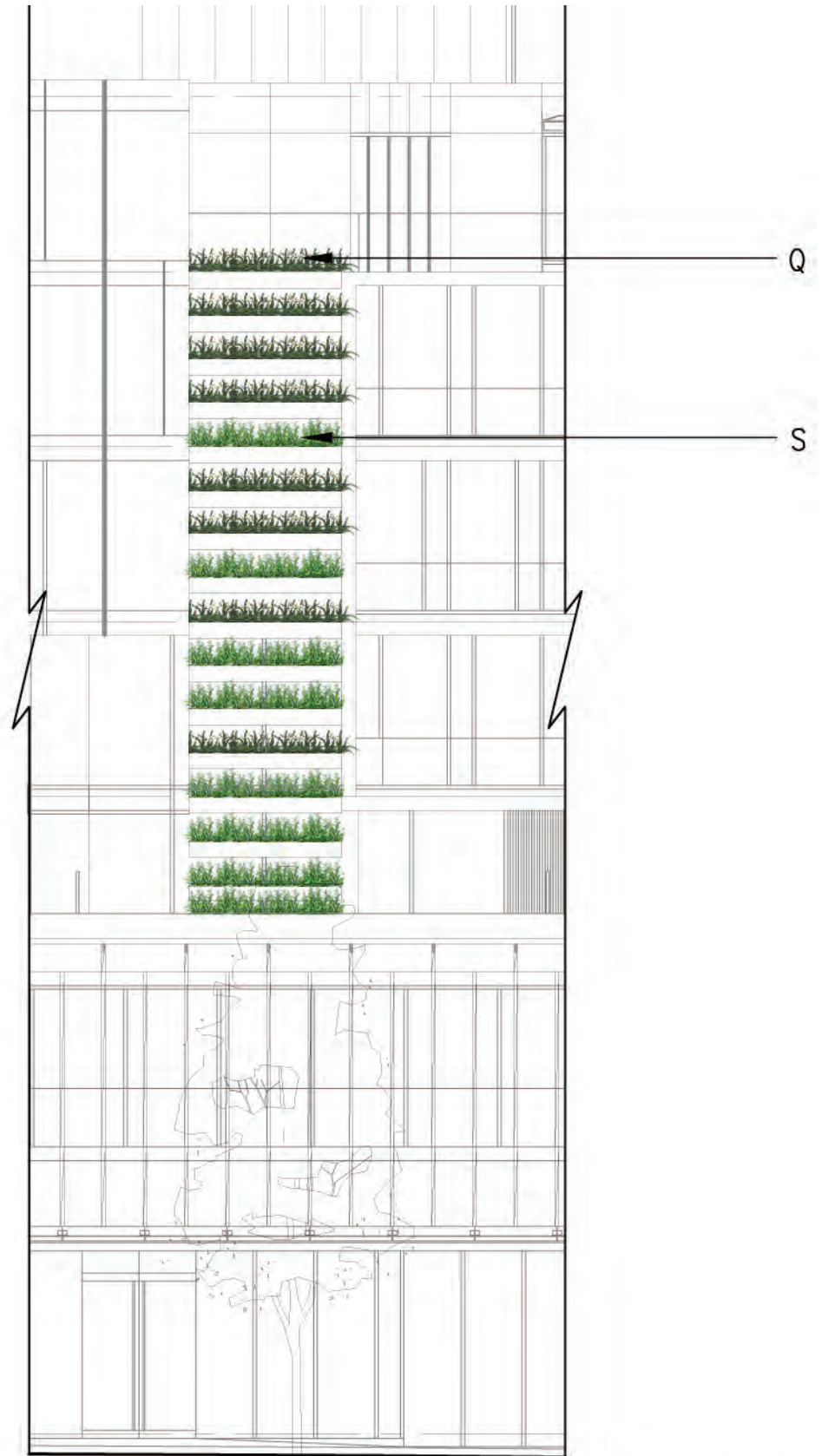
B GREEN SCREEN AT MARINE DRIVE (EAST) 1"=10'-0"
