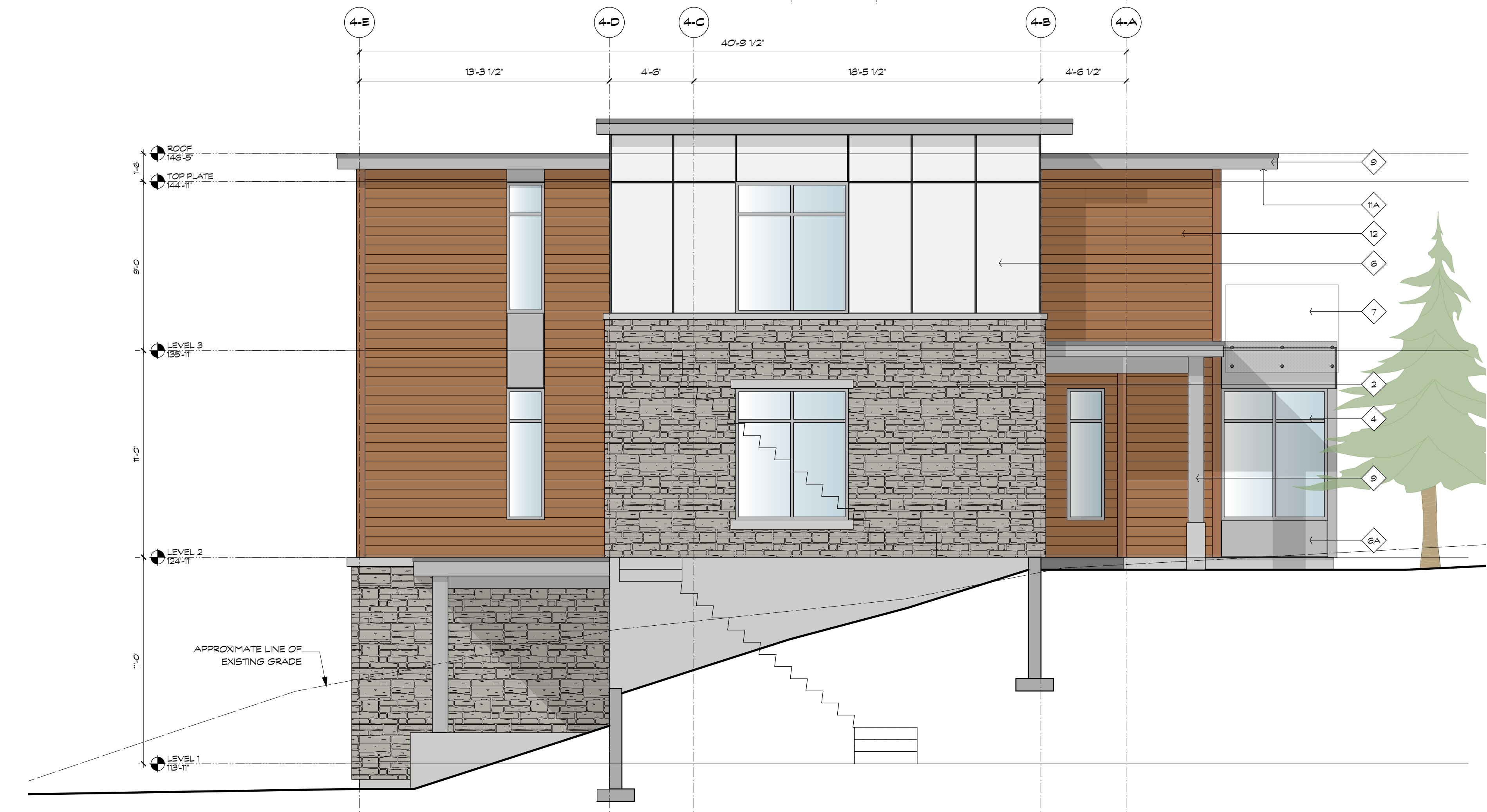
4 HOUSE 4 - SIDE ELEVATION (NORTH) SCALE: 1/4"=1'-0"
