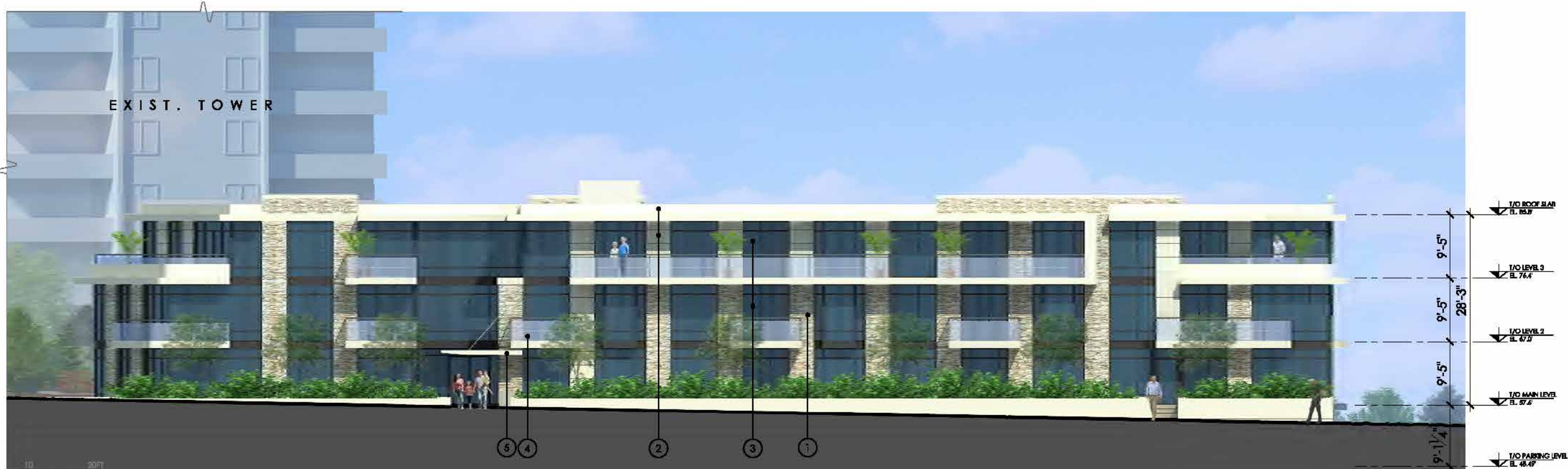
BLDG 'B' NORTH ELEVATION (BELLEVUE AVE.) SC. 1/16" = 1'-0"
