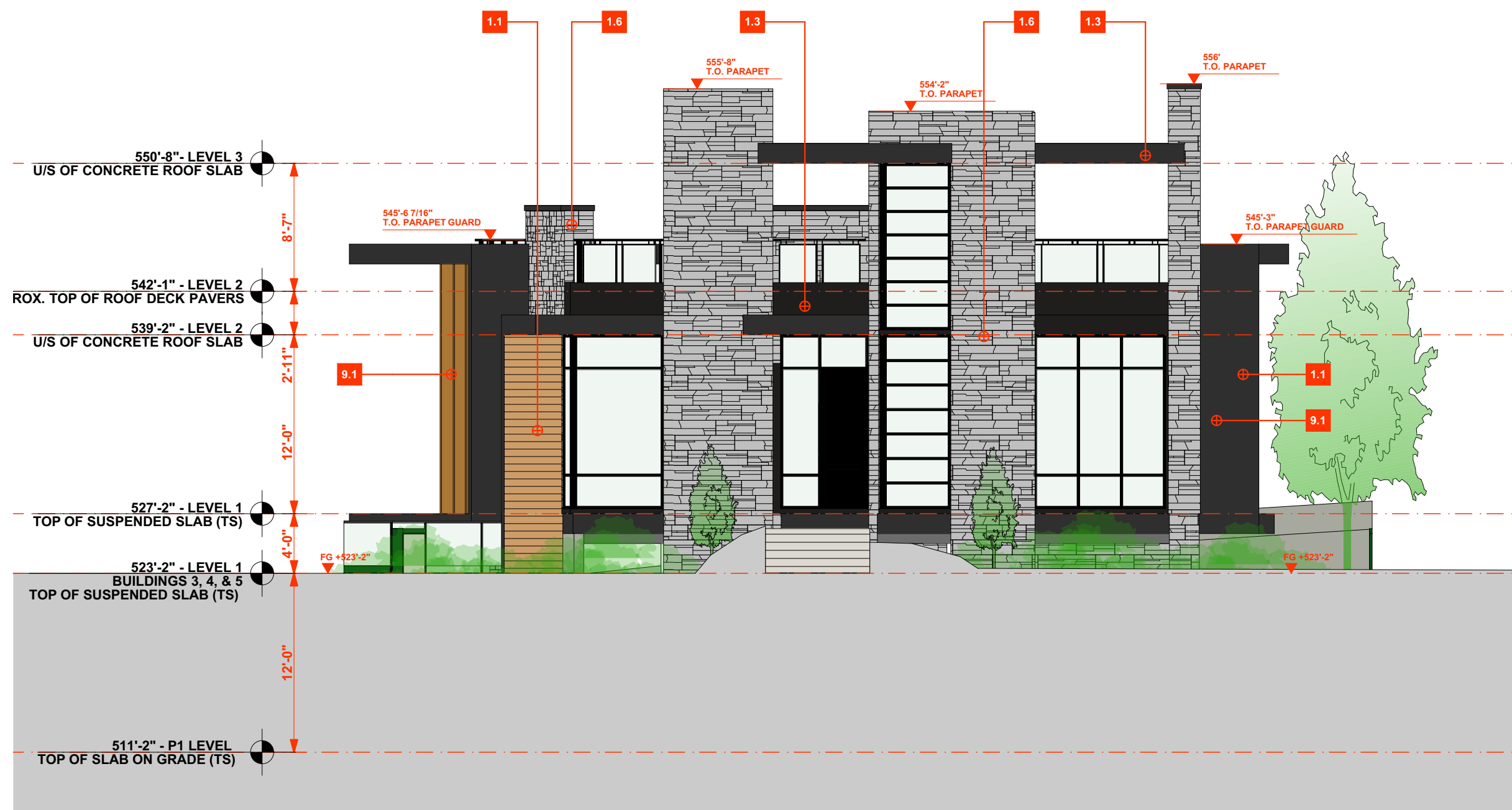
1 Amenity Building - Courtyard Elevation SCALE: 1/8" = 1'-0"
