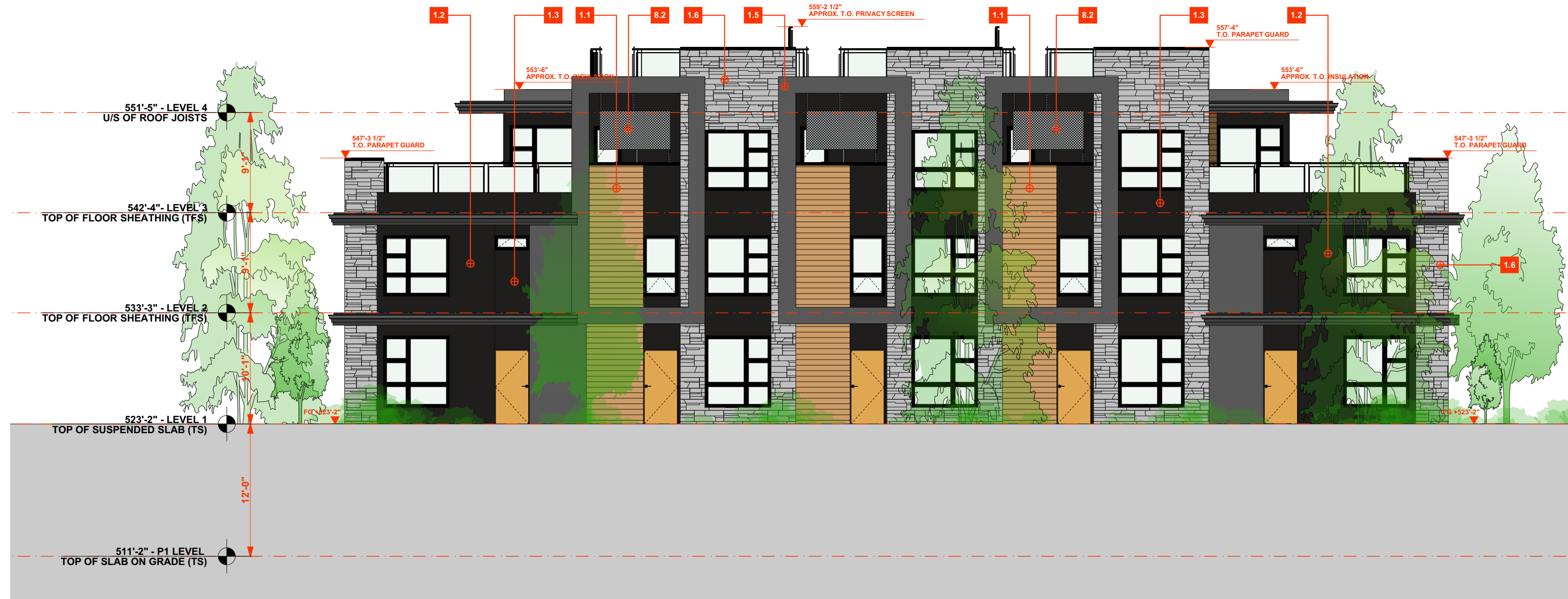
1 Building 3 - Courtyard Elevation SCALE: 1/8" = 1'-0"
