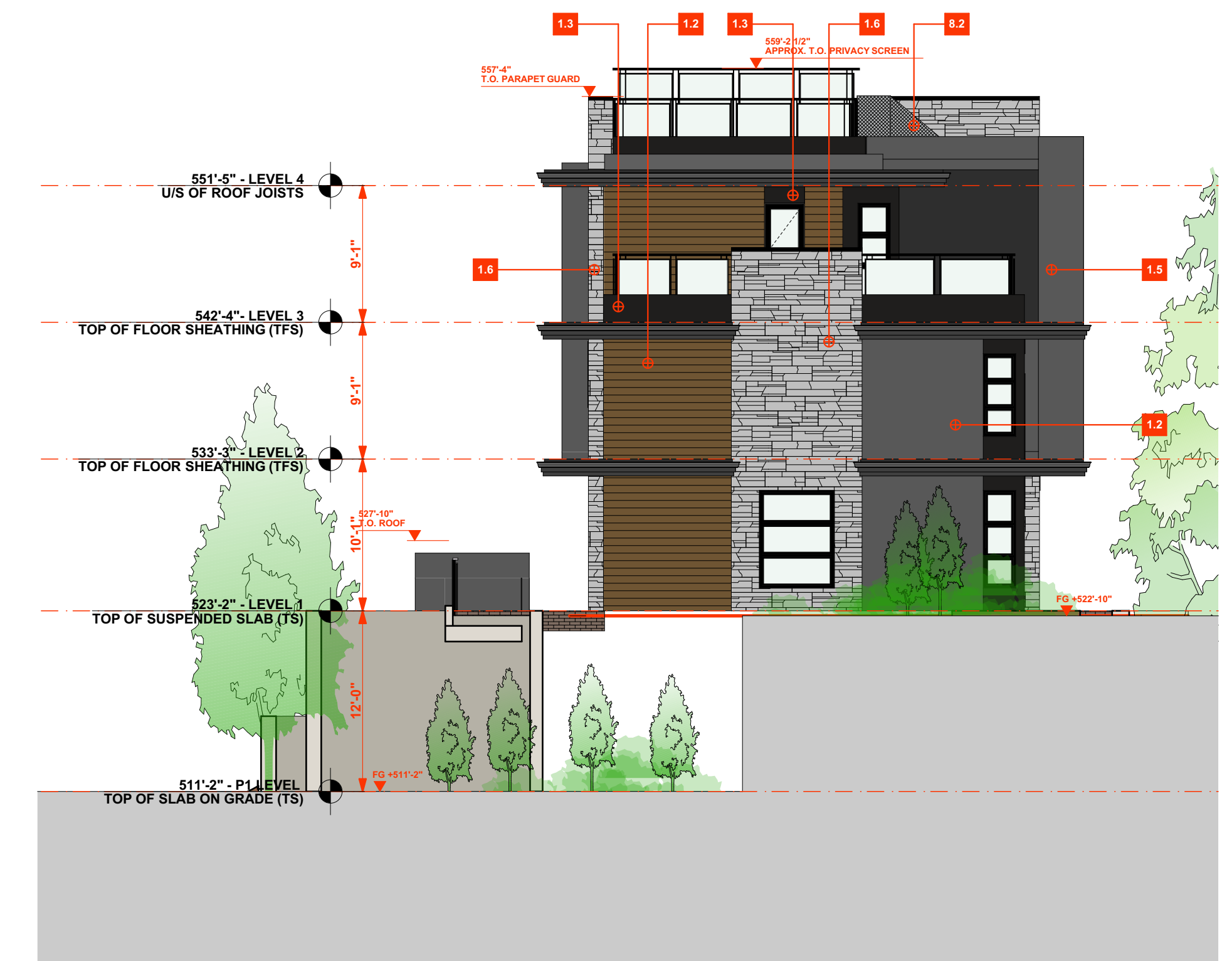
4 Building 3 - South Side Elevation SCALE: 1/8" = 1'-0"
