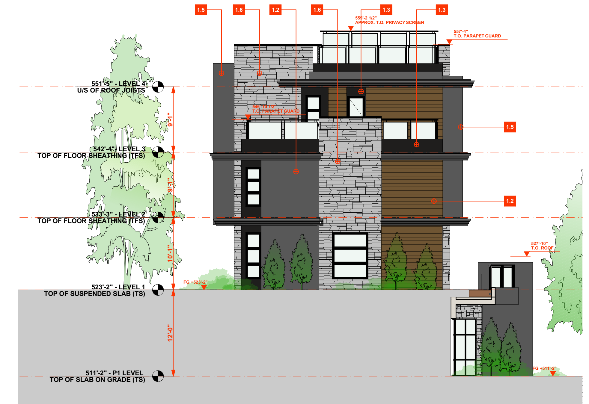
2 Building 3 - North Side Elevation SCALE: 1/8" = 1'-0"
