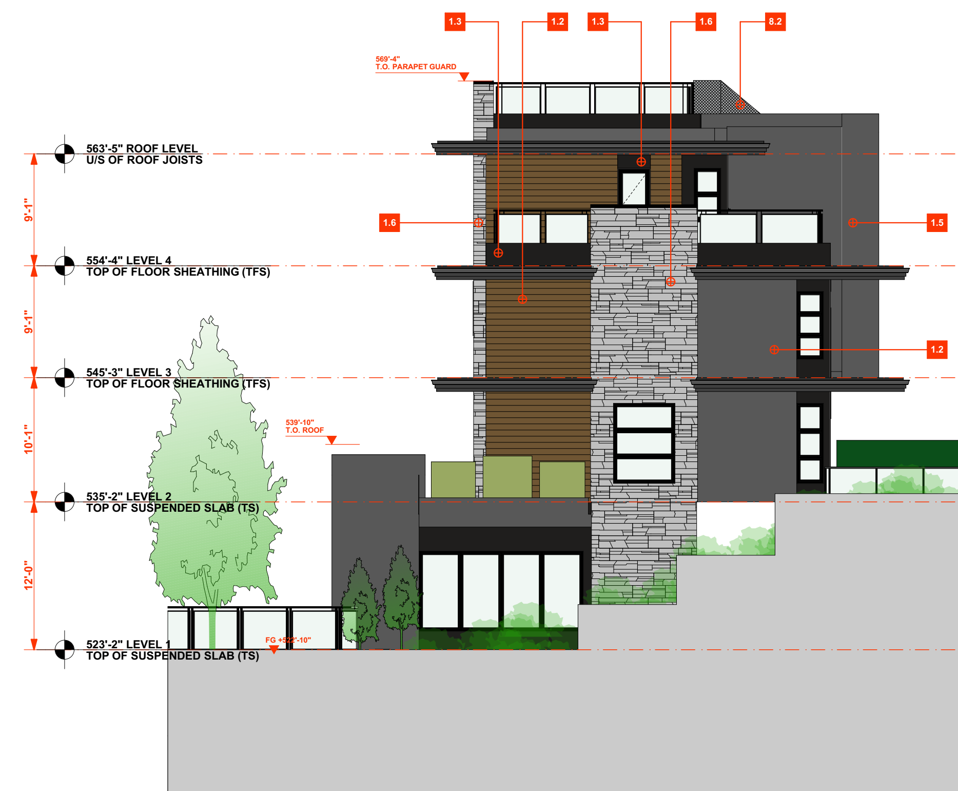
4 Building 2 - South Side Elevation SCALE: 1/8" = 1'-0"
